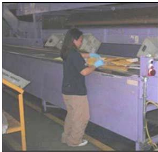
Before – Height of the conveyor results in working above elbow height
