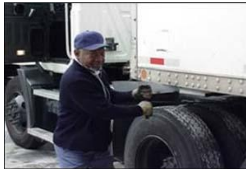
After - Using a tool to pull the 5th wheel release
