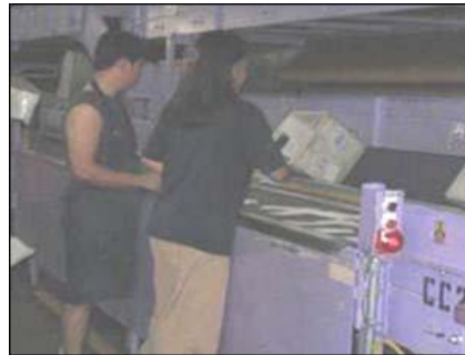
After - Use of a portable platform allows work to be performed at elbow height. Platform has a yellow border to improve visibility and is portable so it can be easily removed
