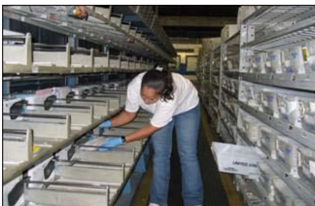
Before – Heavy mail volume falls to the bottom bin resulting in frequent bending and twisting while removing the mail from the machine
