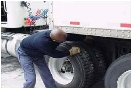
Before - Reaching under the trailer to pull the 5th wheel release
