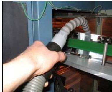
After - Flexible nozzle allows operator to vacuum equipment with a straight wrist
