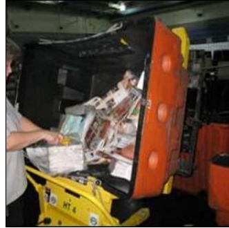
After - Container tilter lifts and tilts the hamper resulting in less bending and reaching
