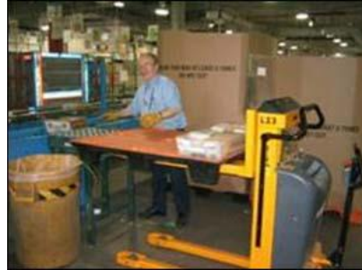
After – Pallet lift allows the person to raise the trays to waist height
