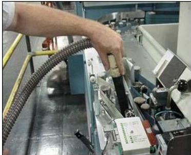
Before - Straight nozzle on the vacuum hose results in awkward wrist and shoulder position to vacuum equipment
